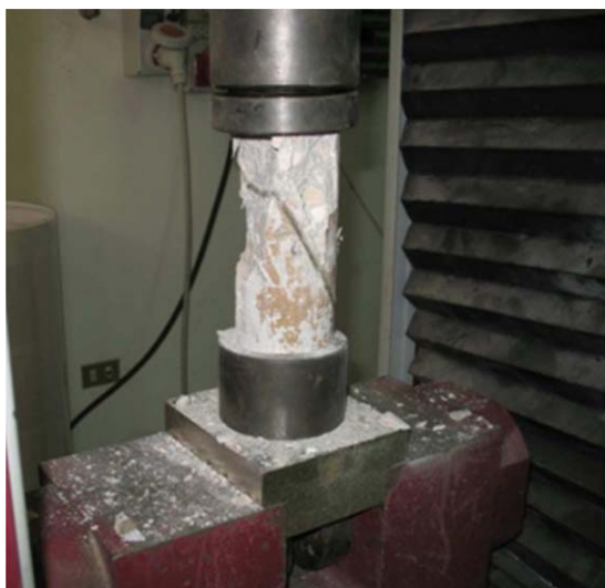
Figure 7. Failure mode in a joint bonded with O-I hybrid resin. [Color figure can be viewed in the online issue, which is available at wileyonlinelibrary.com .]
