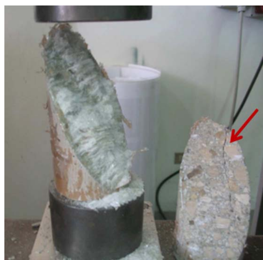
Figure 6. Failure mode in a joint bonded with control resin; the arrow indicates the fracture inside concrete. [Color figure can be viewed in the online issue, which is available at wileyonlinelibrary.com .]
