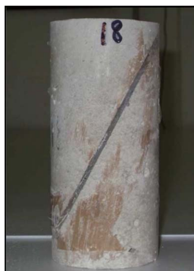
Figure 2. Concrete/concrete adhesive joint specimen after adhesive setting. [Color figure can be viewed in the online issue, which is available at wileyonlinelibrary.com .]
